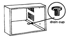
**1** Place drain cup through hole in cabinet rail as shown.
